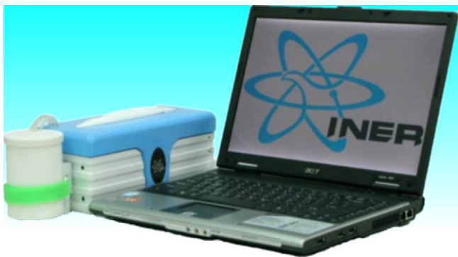
Fig. 13. A notebook PC powered by a portable DMFC system.
